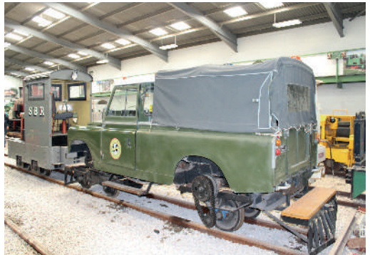
One for Allister! Land Rover Series 2 LWB converted to run on 2ft gauge
