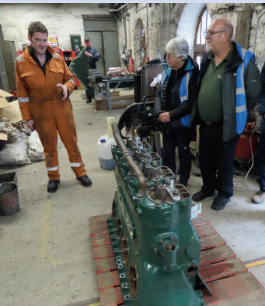
A very rare McLaren MDB4 diesel engine was of great interest. When restored this will power Kerr Stuart locomotive 4415, of 1928 vintage. [SW]
